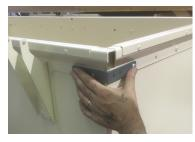
**5.** Install the four corner brackets on each of the top corners of the bin. Using four 1/4" x 3/4" carriage bolts per corner bracket,
