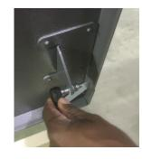
the attachment fairly easily. Once the lower end is installed, extend the gas shock rod out most of the way with your hands. Carefully close the lid until the shock attachment on the lid lines up with rod end of the shock and snap the shock in place the same way.
