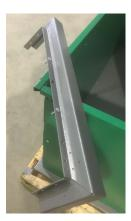
1. Place two  $1/4" \ge 1"$  carriage bolts into two centre holes of one of the Bear Guard Brackets. *(See Image 1)*
